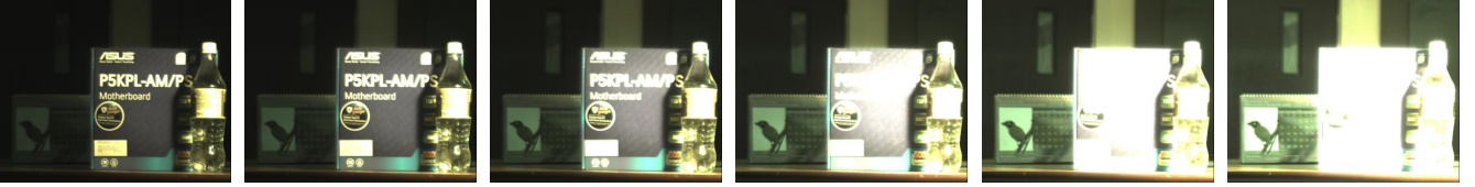
Fig. 3. Gain-shifted images of a bottle placed on a table in an unevenly illuminated environment using firmware approach. The gain ranges from 2 dB to 24 dB at a linear increment of 4 dB.
